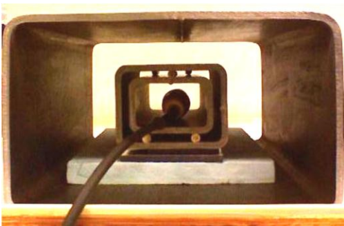
Fig. 1. The three layers of magnetic shielding. The Narda EFA-300’s MF probe is in place of the culture vessel. MF coils for exposure are below, but not in contact with the two smaller shields, insulated from the outer shield by a layer of rigid foam.
