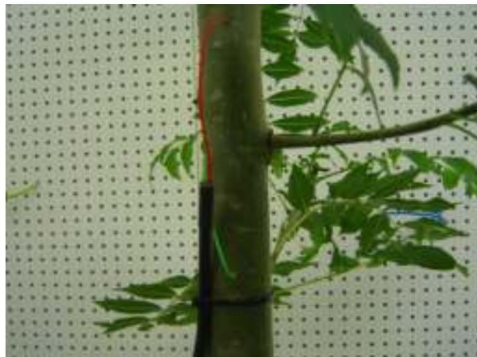
Figure 2 Flash-gold plated electrodes
