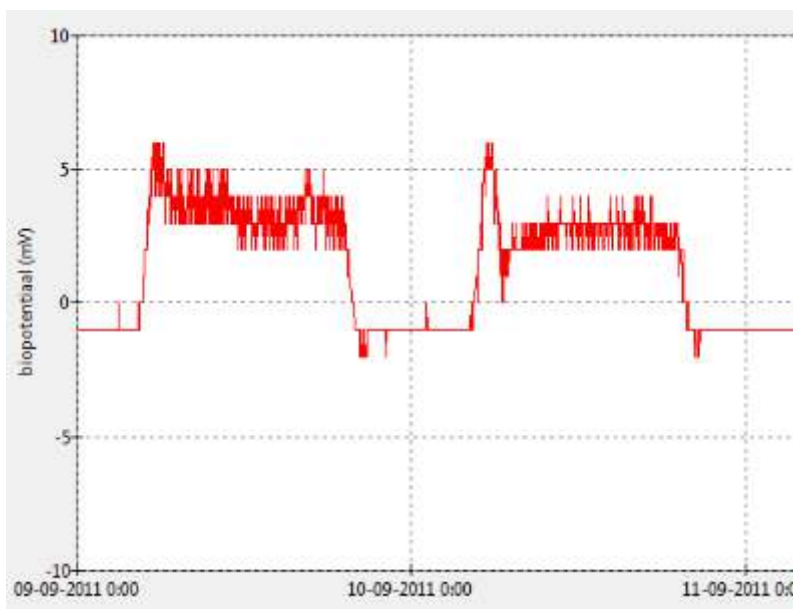
Figure 10 Measurements on plane timber wood with WiFi stations activated
